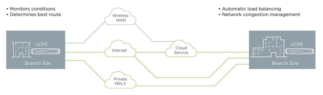
SD-WAN dynamically sends traffic over multiple WAN connections to create cost savings and application efficiency.
