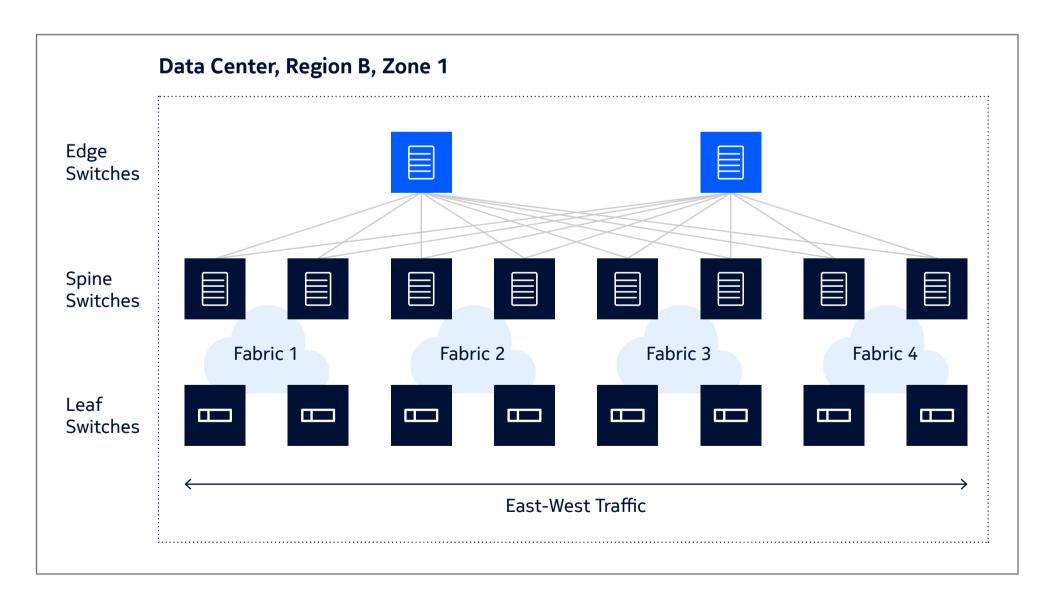
A greater number of network devices that require configuration and management is driving a change in how data center networks are designed in order to provide greater bandwidth within and between data centers.
