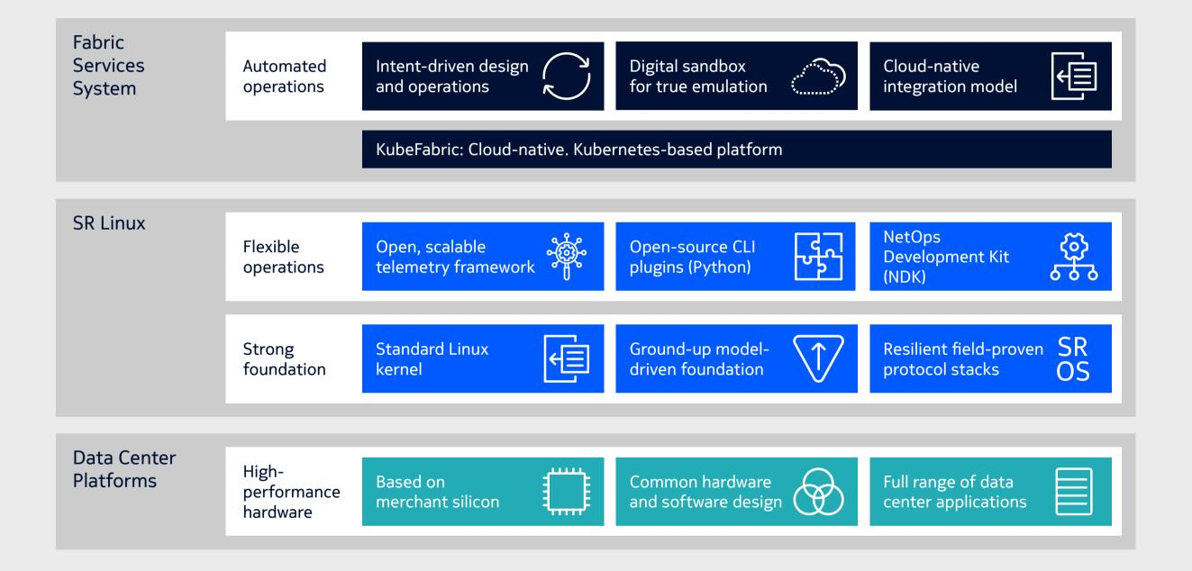
The next-generation Nokia Data Center Fabric solution has been designed from the ground up to free your cloud builder networking teams to rapidly design and deploy, easily adapt and integrate and confidently operate and automate data center network fabrics: at scale. Nokia brings together the following products in one new era-redefining solution:
